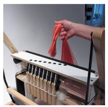
When it's completely wound on, remove your elastic and take the warp threads out of the raddle.
