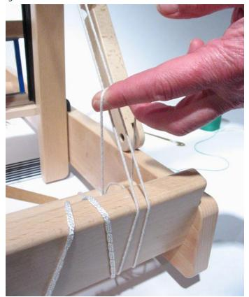
Cut two cords about 2yds long. Half-hitch one on the right side on the back beam as shown in the picture. Then half-hitch the other on the left side of the back beam. These will be used to suspend the lease sticks from the back beam to the beater arms.
