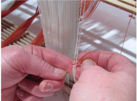
Here I am threading the heddles. Take a look at the video for a good closeup of the threading technique and tips about Texsolv heddles.
