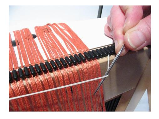
Place an elastic band over the raddle to prevent threads from escaping.
