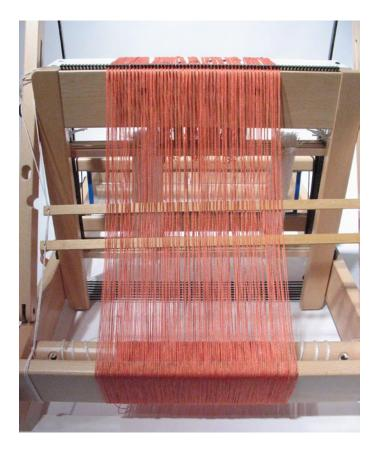
Here you can see that the warp is winding on evenly at the proper width.
