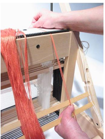
Thread your raddle directly from your cross. **Important**: if you have warped with more than one thread, never split those thread groups going through the raddle. Example: if you have warped with three threads in your hands, keep those threads all together.
