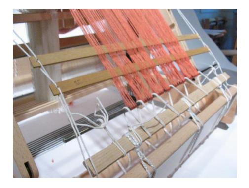
The lacing cord such as heavy seine twine is now in place, laced around both rods approximately every 2".
