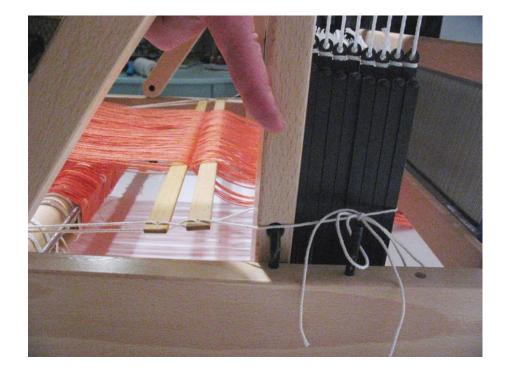
Here the position of the cords that hold the lease sticks has been changed. They have been brought down from the beater arms and tied around the entire castle. This allows easier access to the cross for threading.
