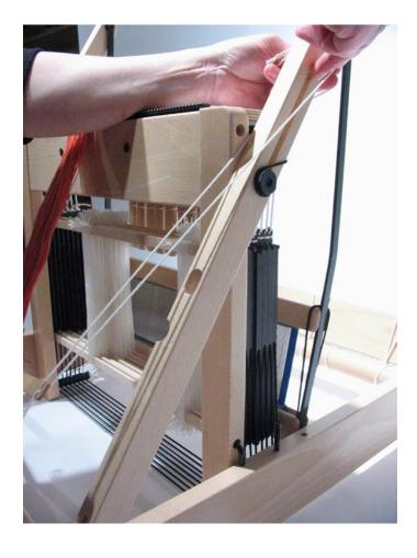
Attach both of these ends around the beater arm and tie them up so they are nice and taut. Your lease sticks will now be suspended between the back thread beam and the beater uprights. The cords should form a nice cross between the lease sticks which will prevent them from moving on top of each other. However, your lease sticks will be able to move and let you know if you have a snag.
